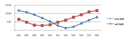
•SMALLEST reads best without any metal bolt in two holes (located diagonal directions). With RF interference, metal bolts decreases read range by 20% or more. RFcamp recommends not using metal bolts, but 3M 300LSE adhesive or glue for maintaining optimum read performance. In case adhesive or glue can not be used, polycarbonate (or nylon) bolts is recommended.
