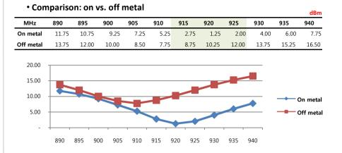
•SMALLEST reads 60% shorter off metal (or on non metal surface). It can be applied, therefore, only for metal application. For non metal application, please use SMALLEST NM.
